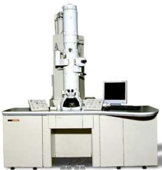
Figura 2. Microscopio TEM JEOL JEM-2100
